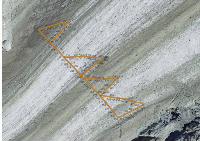
Estimated channel locations of the fiber optic cable on Otemma Glacier, Valais, Switzerland.
